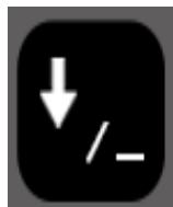
Downward navigation button. When BATCH is on, press to choose 10/20/50/100.
